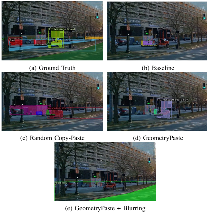
Fig. 5: Visualization of results obtained from the model trained for 30k iterations. Only GeometryPaste detected the TTC Message Board.
